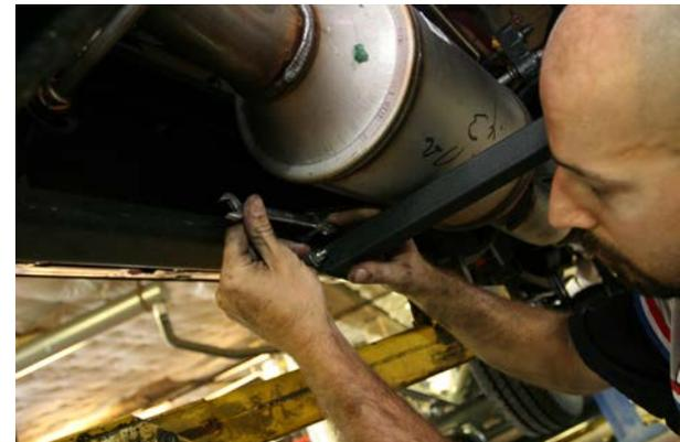
(Fig. 10) Tighten cross member against frame using 5/16" plated bolts, washers and nylon locking nuts provided. Note exhaust particulate filter above cross member.
