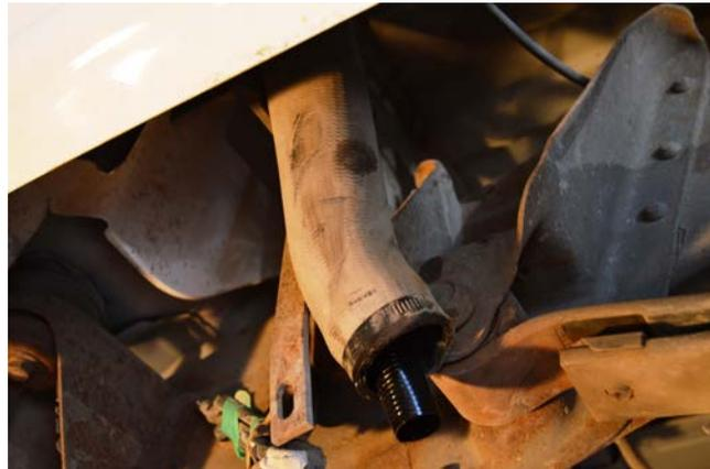
(Fig. 14) On vehicles with LB7 engines only, an interior fill hose is located inside the main fill hose. The tank vents through the space provided between the two hoses. Ten (10) inches needs to be cut off of the interior hose on end that goes to the tank as shown.
