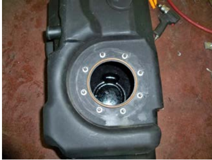
(Fig. 3) Leave the “O” ring gasket, studs and retainers assembled as they are (shown before sending unit, top flange, and 3/8” nylon Locking nuts are installed).
