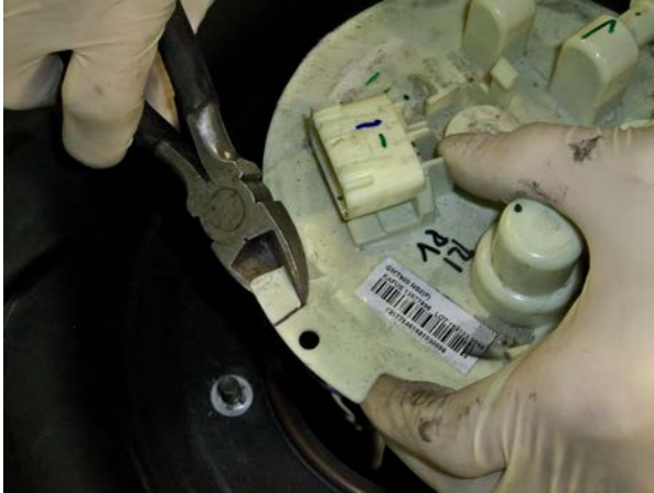
(Fig. 5) If sending unit connections interfere with the mounting studs, trim ½" off the side of the tab nearest the electrical connector.
