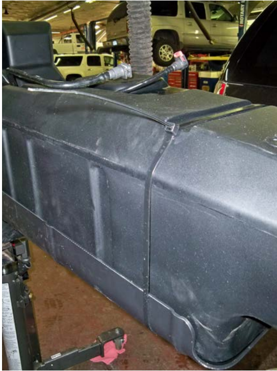
(Fig. 11) Use Quick Tie to fasten shield at front of tank at indentations. Cut off extra.
