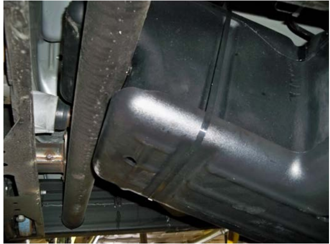
(Fig. 12) Angle front of tank up and over round tubular steel cross member.
