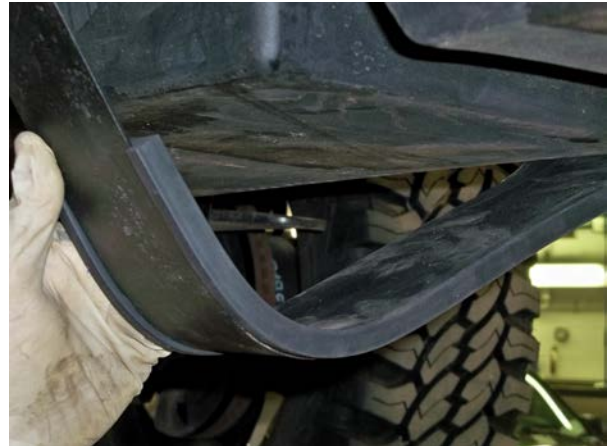
(Fig. 14) Rubber bushings installed on straps when optional TITAN Shield is not used.
