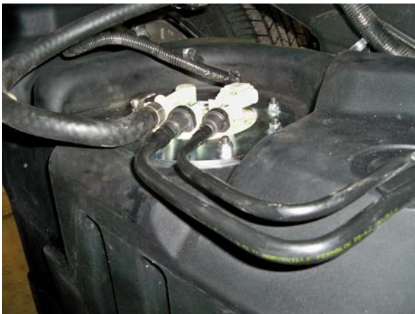
(Fig. 13) Lift tank high enough to reconnect electrical cable and vent hose to sending unit.
