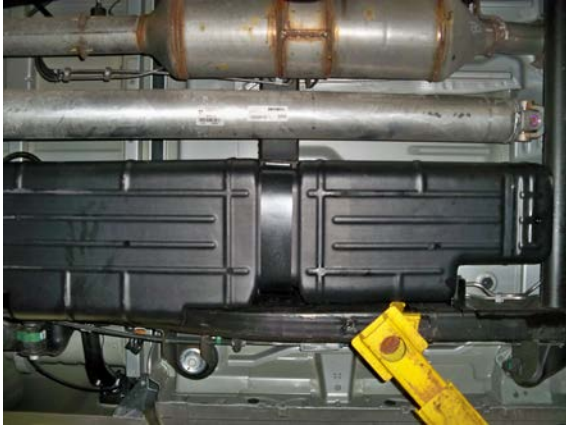
(Fig. 15) Installation showing optional TITAN Shield.
