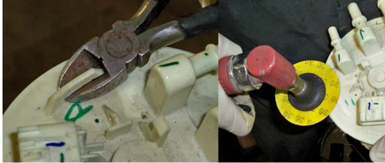
(Fig. 4) If sending unit is equipped with curved ribs on the top, either shave approximately 1/16” off the outside surface of both, or remove the rib closest to the electrical plug using dikes and a hand grinder-sander as shown above so top flange will fit correctly. Be sure surface is perfectly smooth and even to prevent breakage when top flange is tightened.
