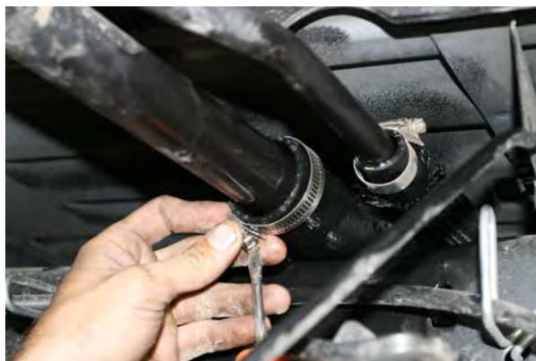
(Fig. 11) Attach fuel tank 1  $\frac{1}{2}$ " fill hose and  $\frac{3}{4}$ " vent hose to vehicle fill spout. On some long-bed tanks, 1  $\frac{1}{2}$ " fill hose may have to be extended with 3.25" hose extension.
