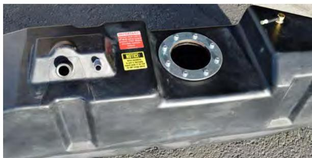
(Fig. 10) Install the OEM 1  $\frac{1}{2}$ " fuel tank fill hose to the large king nipple and the  $\frac{3}{4}$ " OEM vent hose to the smaller nipple. Be sure to fasten tightly with the OEM hose clamps.
