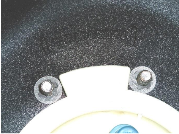
(Fig. 3) Line sending unit tab up with “TAB LOCATION” marks on tank.
