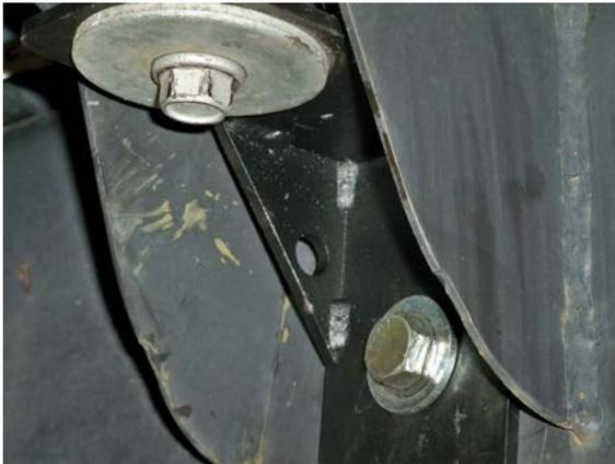
(Fig. 11) As an alternative to drilling the frame, the cab mount gussets can be drilled in-line with the "S" Bracket gussets and bolted into place. See the holes in the bracket gussets shown above.
