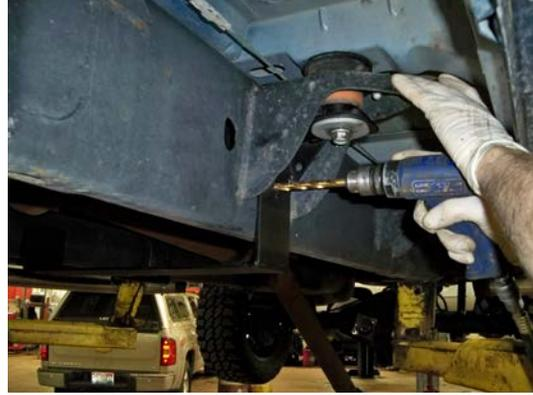
(Fig. 10) This shows the "S" Bracket Support bolted to the cab mount below the driver's door. As shown, drill a hole through the vertical center-hole of the bracket and fasten with the bolt provided.
