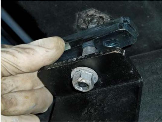
(Fig. 13) Thread two shims onto each strap bolt.
