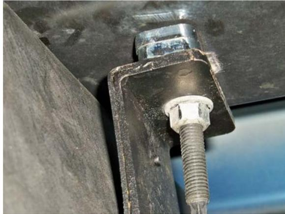
(Fig. 14) Tighten the bolt and bracket against the shims. If the strap does not hold the tank tightly enough, remove one shim at a time until it is tight.
