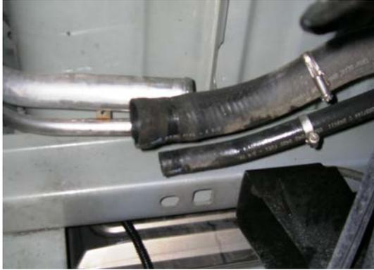
(Fig. 1) Disconnect 1 ½” fill hose and ¾” vent line from fill spout leaving them attached to OEM tank.
