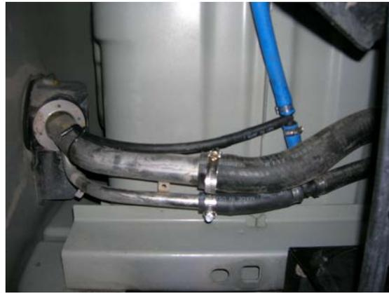
(Fig. 8) Photo shows final installation of fill hose and vent line hoses on vehicle's fill spout. Note the ¼" Vent Kit Assembly hose is securely fastened to the fill spout. The ¼" vent is necessary to prevent vacuum build-up in your TITAN™ fuel tank.
