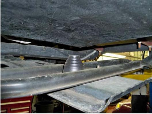
(Fig. 9) This photo shows the Cushion Mount installed on the factory skid plate below the tank.
