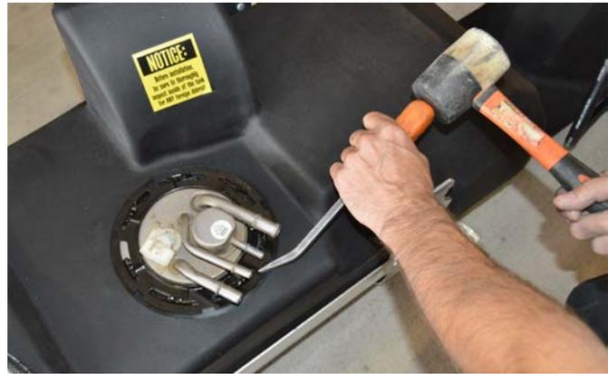
(Fig. 4) Tighten the provided TITAN Torque, hold-down ring by turning it clockwise as far as it will go.
