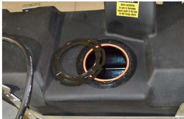
(Fig. 2) TITAN sending unit mounting hardware before sending unit is installed.
