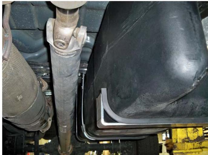
(Fig. 12) Installation of front support on tank without TITAN Shield. Note the flexible bushings on the support and the straps.
