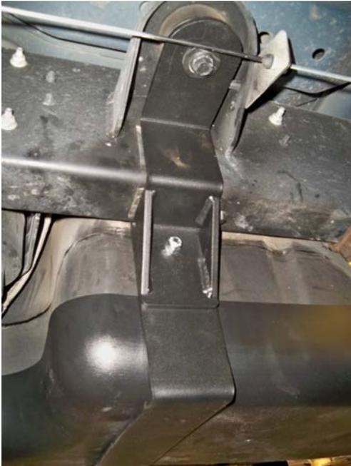
(Fig. 11) Completed front support installation on tank with TITAN Shield.
