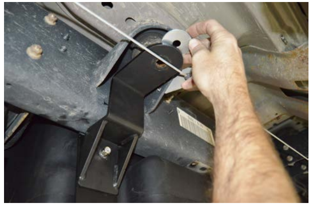
(Fig. 8) Place the supplied fender washer into the center of the rubber cab mount above the upper piece of the assembly.
