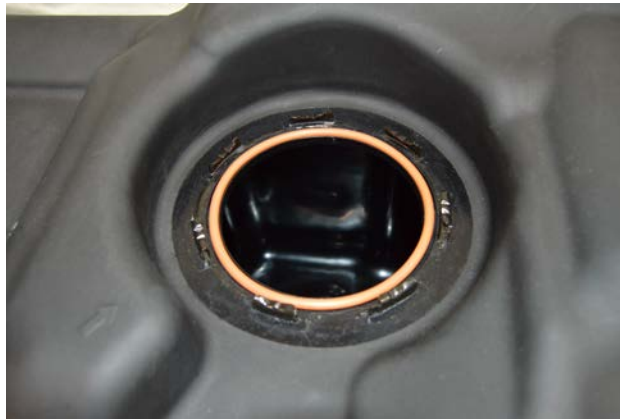
(Fig. 3) O-Ring gasket shown installed correctly.
