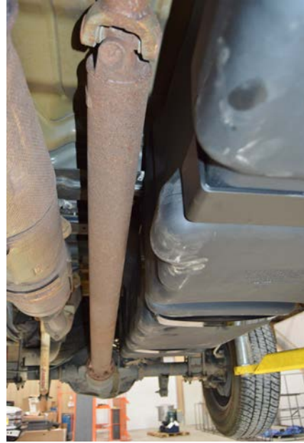
(Fig. 12) Installed front support on tank.
