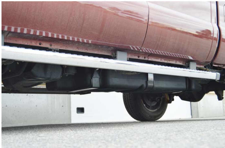
(Fig. 11) Completed front support installation and tank.
