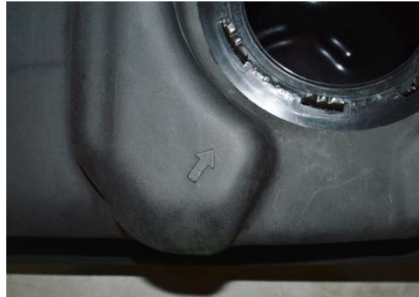
(Fig. 4) Line the sending unit tab up with the tab location arrow marking on the tank.
