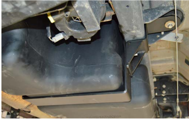
(Fig. 11) Completed front support installation and tank.
