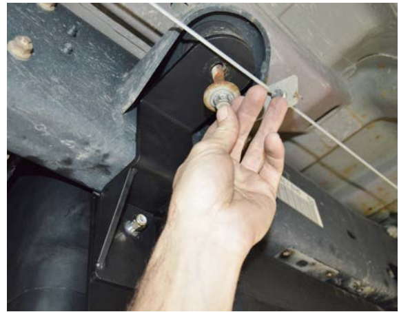
(Fig. 10) Replace cab mount bolt with its existing washers and tighten to factory specification.
