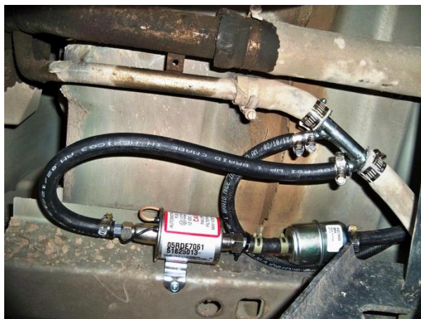
(Fig. 15) Vent Fill Neck Adapter installed.
