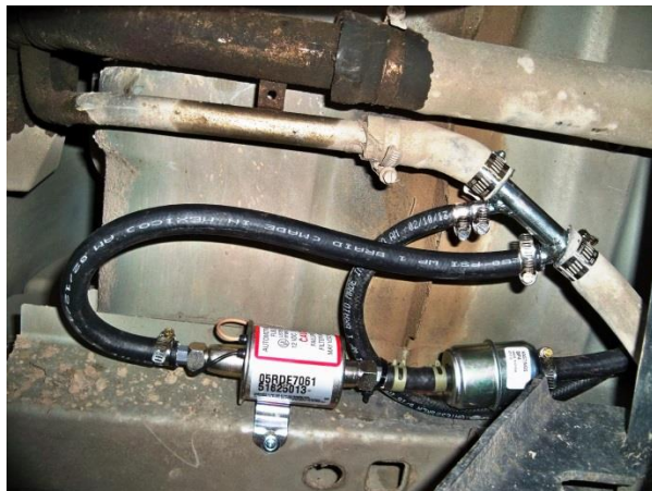
(Fig. 15) Vent Fill Neck Adapter installed.
