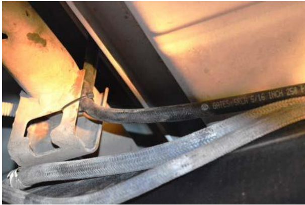
(Fig. 7) One of the vent hoses routed up and attached to the vehicle's body with quick tie.
