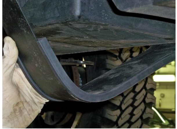
(Fig.13) Extruded bushings installed on straps
