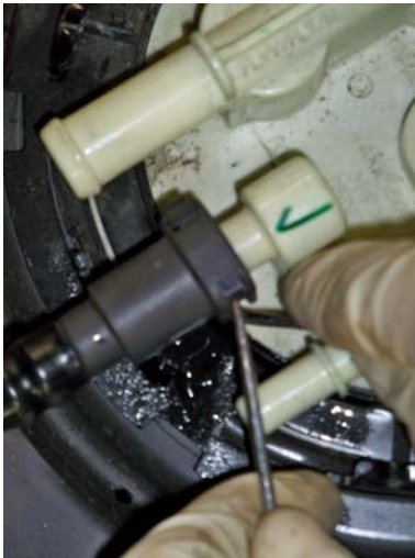
(Fig.2) Disconnect fuel lines at the sending unit using pick.
