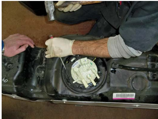
(Fig.3) Loosen hold-down ring on OEM tank by tapping counter-clockwise, remove and lift out sending unit.
