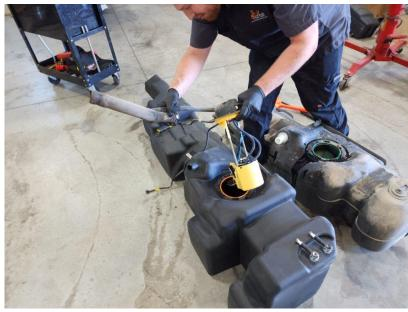
Make sure the tab on the sending unit is lined up with the "Tab Location" mark on the TITAN tank.
