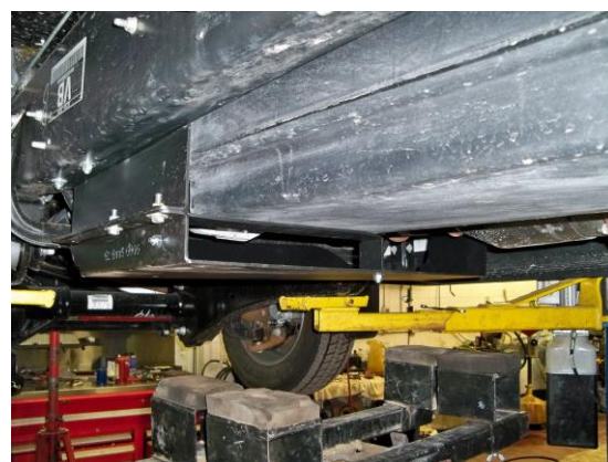
(Fig. 6) Skid plate bolted into place on bottom of formed channel. Note Nose Bracket is in "high" position.
