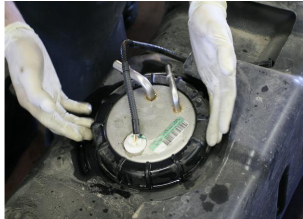
(Fig. 2) Remove the sending unit from the original equipment tank by rotating the hold-down ring counter clockwise.
