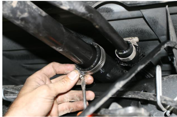
(Fig. 12) Attach fuel tank 1 \frac{1}{2} " fill hose and \frac{3}{4} " vent hose to vehicle fill spout. Vent hose may have to be shortened about 6 inches to fit properly. On some long bed tanks, 1 \frac{1}{2} " fill hose may have to be extended with 3.35" hose extension.
