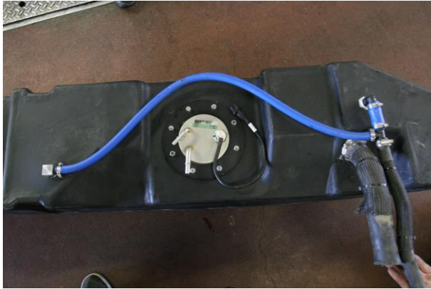
(Fig. 11) Top view of SHORT BED tank showing sending unit, tank vent hose plumbing, and original equipment fill hose and vent hose installation. The \frac{1}{2} " x \frac{1}{2} " x \frac{1}{4} " tee is not shown installed in the \frac{1}{2} " vent line hose. It will be installed approximately 2" from the rollover vent valve.
