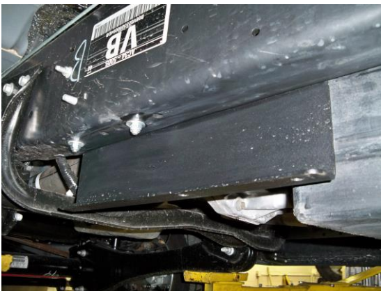
(Fig. 5) Formed channel is bolted to the inside of the frame on the driver's side.
