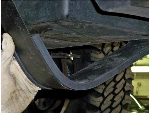
(Fig. 5) Install rubber bushings (pn 99 0000 0103) on both straps with the channel side toward the strap.
