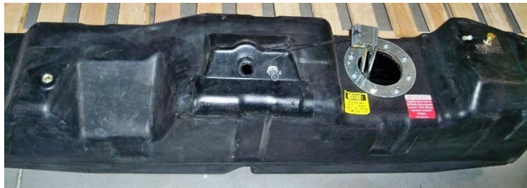
(Fig. 4) This photo shows the venting accommodation for the tank. Use the stock tank's fill and vent hose to attach to the king fill and vent nipples shown in the center. No additional hose is needed. This is how the tank comes out of the box.
