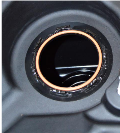
(Fig. 3) O-Ring gasket shown installed correctly.
