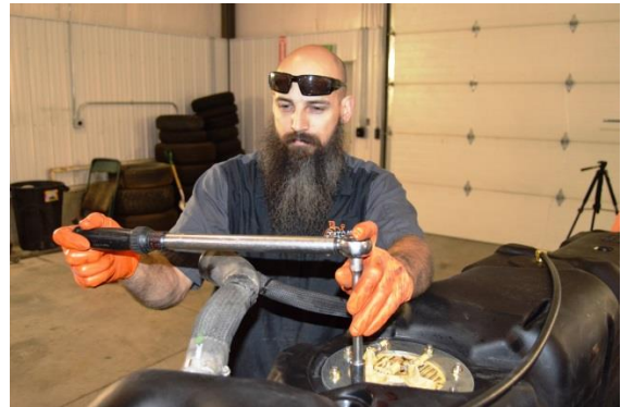
(Fig. 3) Place the sending unit into the TITAN tank, install the top flange, and tighten the nylon lock nuts to 20 ft. lbs using a “star” pattern using a torque wrench.
