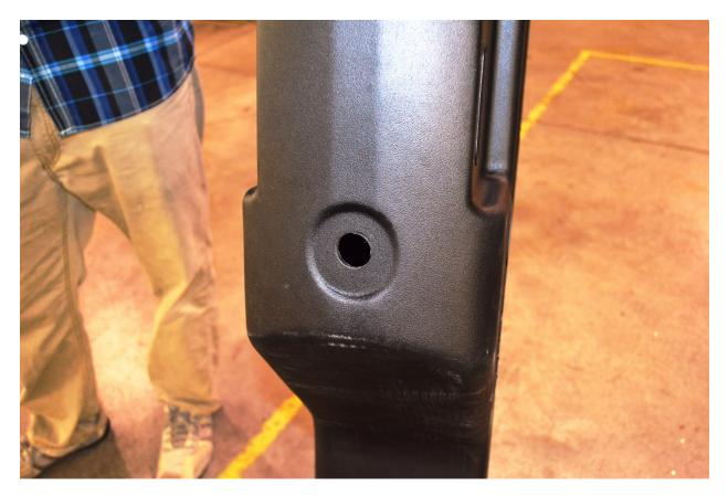
2 Thread the chain and plug weldment through the bulkhead fitting as shown below. Screw plug loosely into the bulkhead fitting.
