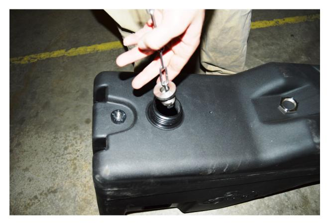
4 Thread bulkhead fitting through hole, install jam nut and remove the chain and plug.
