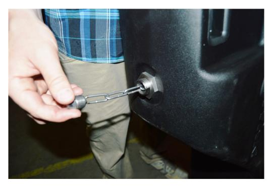
5 Tighten jam nut using spanners.
