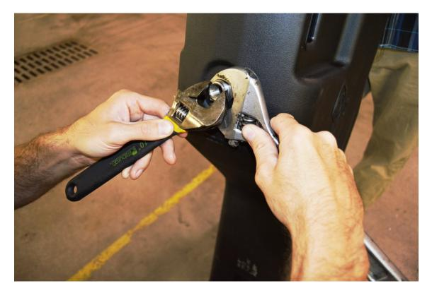
6 Install and tighten 3/8" NPT Hex Socket Plug, if desired, and installation is complete.
