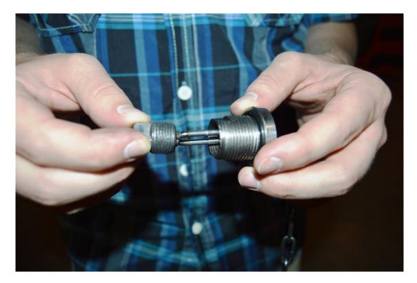
**3** Drop bulkhead assembly through fill neck on chain as shown.
