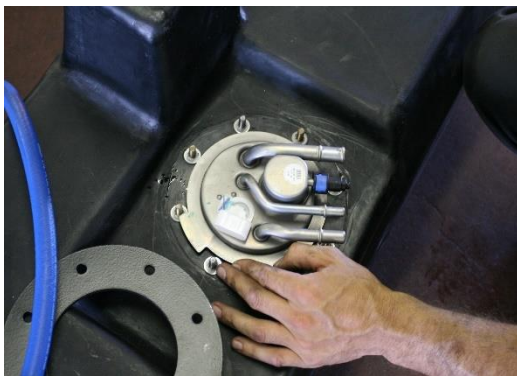
(Fig. 5) Make sure fuel line fittings point at the same angle as in original equipment tank.
