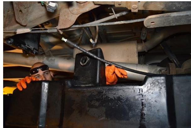
(Fig. 8) The ends of both vent hoses must be installed higher than the tank's fill tower. Front vent hose is shown here.
