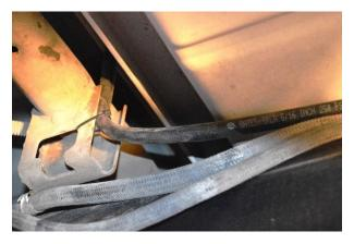
(Fig. 9) One of the vent hoses routed up and attached to the vehicle's body with quick tie.
