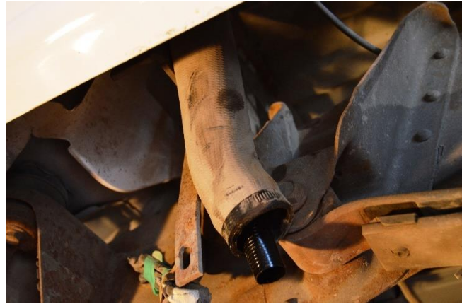
(Fig. 12) On vehicles with LB7 engines only, an interior fill hose is located inside the main fill hose. The tank vents through the space provided between the two hoses. Ten (10) inches needs to be cut off of the interior hose on end that goes to the tank as shown.
