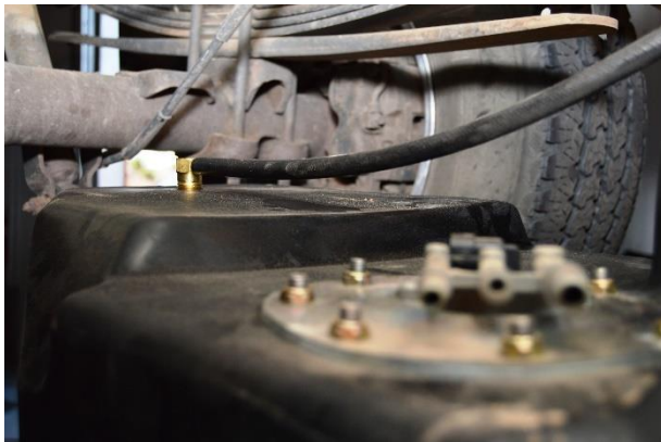
(Fig. 7) Rear rollover valve with vent hose attached.
