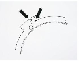
(Fig. 4) Diagram showing where to trim sending unit tab. Cut the tab along the dotted line as shown above using a pair of diagonal cutters, a hack saw or a grinder.
