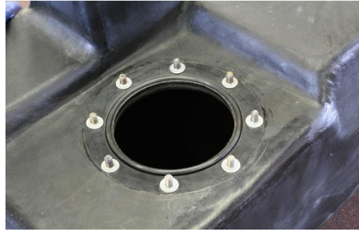
(Fig. 2) Sending unit mounting hardware before sending unit, top flange, and 3/8” nylon locking nuts are installed.
