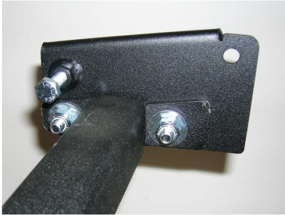
(Fig. 11) Shown: Right-Hand Bracket for GM Cross Bar. The Cross Bar is held fast by tightening the 5/16" cap screw seen here at the upper left hand corner of the bracket. It is recommended that the installer position the Cross Bar, tighten down the cap screw as shown, and then drill a hole in the frame lip through the hole seen in the right-hand corner of the bracket. A 5/16" cap screw and nylon locking nut are provided for fastening this hole. It is advisable to apply Loctite Thread locker or equivalent to the bolts.
