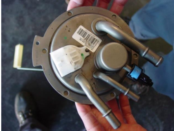
(Fig. 3) New GM sending unit showing tab which, in some cases, interferes with mounting studs in the TITAN Tank. If the tab interferes, it will need to be trimmed.
