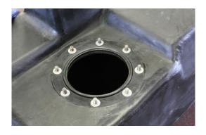
(Fig. 2) Sending unit mounting hardware before sending unit, top flange, and 3/8" nylon locking nuts are installed.
