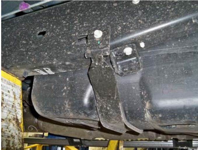
(Fig. 1) Remove original equipment strap and “bumper bracket”, shown here to the right-hand side of the front strap.
