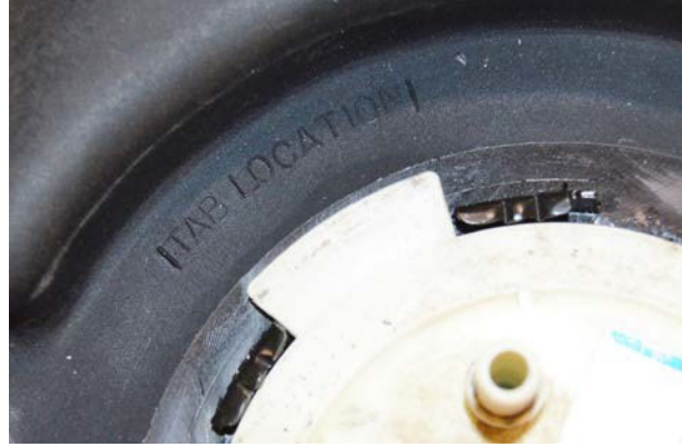
(Fig. 4) Line the sending unit tab up with the "Tab Location" markings on the tank.
