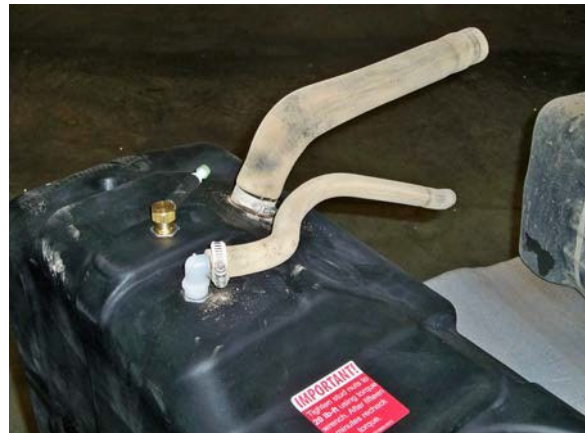
(Fig. 6) Install fill and vent hoses from original equipment tank on TITAN tank as shown. Make sure that \frac{3}{4} " vent line is lined up with orientation mark on the tank.
