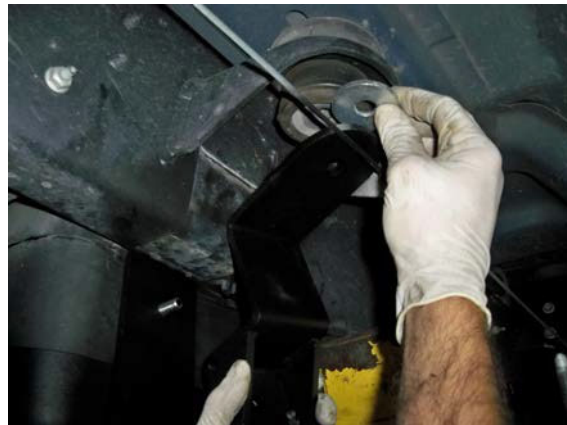
(Fig. 8) Place the supplied fender washer into the center of the rubber cab mount above the upper piece of the assembly.
