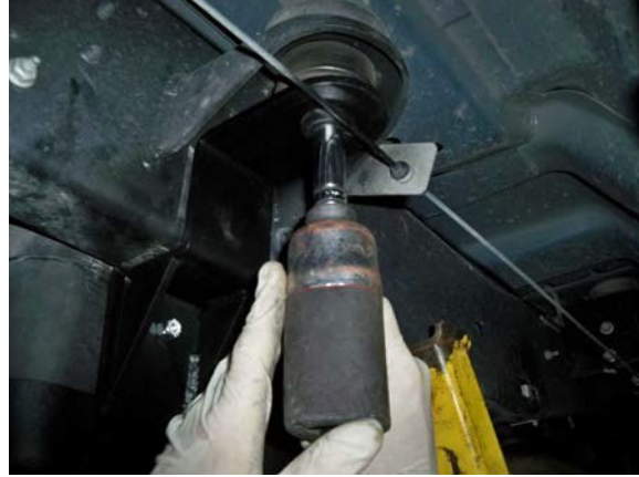
(Fig. 10) Replace cab mount bolt with its existing washers and tighten to factory specification.
